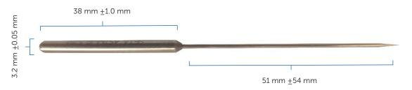
[ASTM: 50 to 55 mm (350 - 500 PEN) IP: > 40 to 45 mm and ferrule must not penetrate (330-500 x 0.1 mm)]
