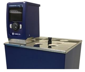
The 35 litre oil bath can accept up to six sets of glassware. The stirred oil is maintained to within  $\pm 0.1$  °C at 95 °C by an integral thermostir unit, that has been designed for continuous use over extended periods, incorporating a stirrer motor well recognized for longevity. The temperature measurement system uses a PT100 probe to ensure long term temperature stability without routine maintenance or re-calibration.
