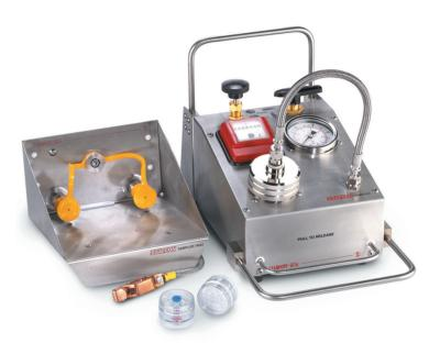
A bypass valve directs fuel through a filter cell containing the removable membrane filter or allows flushing of the sampler. Tested fuel may be routed to a flow line leading to a dump tank, without the need for buckets or containers.
