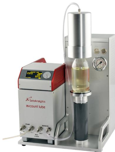
AvCount Lube comprises two modules; the Sample Delivery System (SDS) and the Particle Counter Module (PCM). The PCM can be used independently from the SDS and computer as a compact portable instrument for testing light lubricants and oils with a viscosity up to 64 mm<sup>2</sup>/s. Up to 600 measurements can be saved in the PCM memory ready for downloading via ProTrend. The PCM has three embedded test methods;
